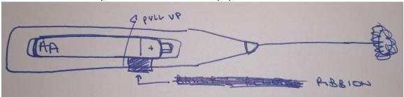
3. Place a new battery in the cavity with the positive side towards the top and the negative side towards the whisk attachment. Push the battery down until you hear a click.
